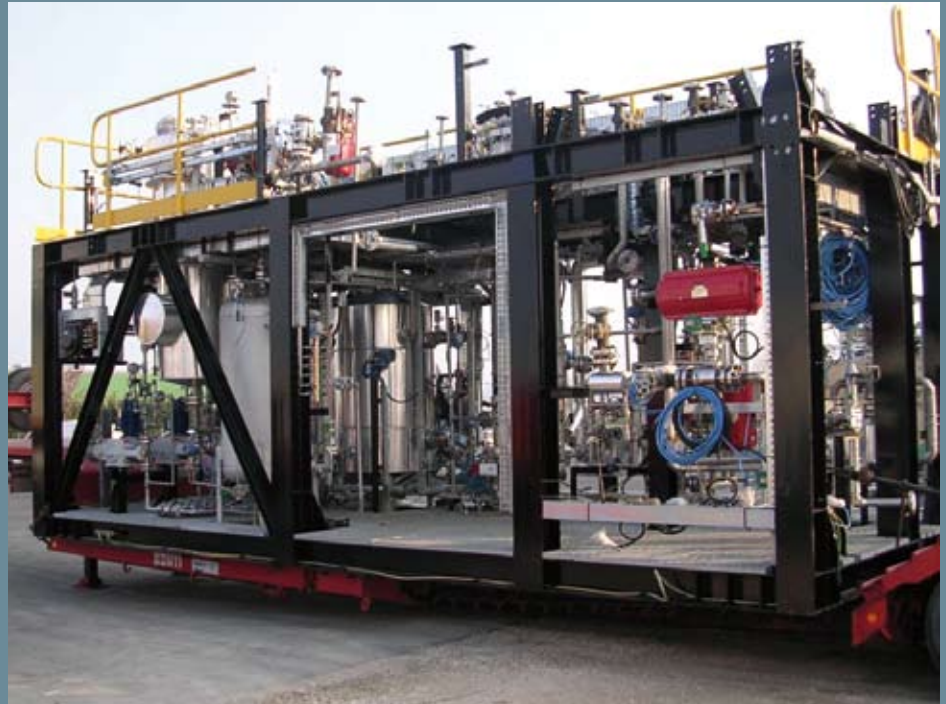
SCT-CPO Process module (street transportable)
