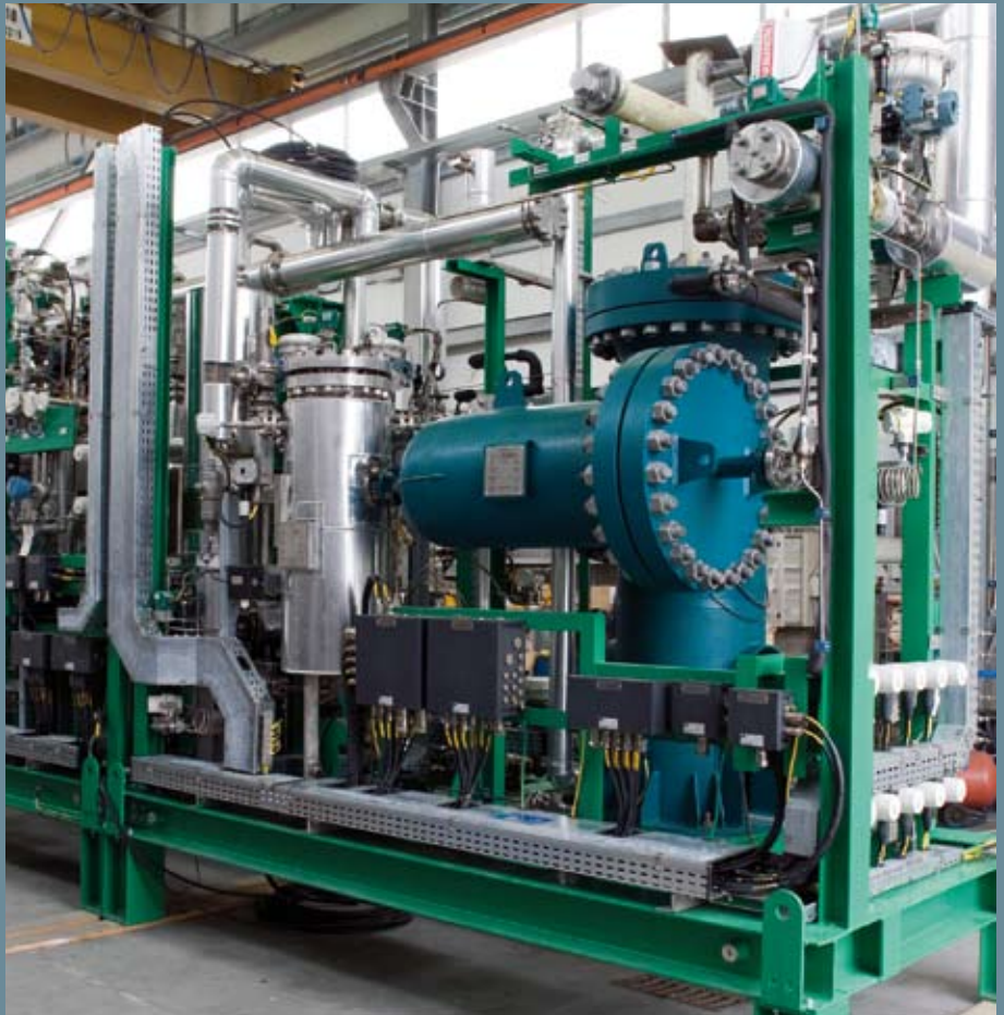
Skid-mounted SCT-CPO Unit (for medium-small hydrogen consumer)
